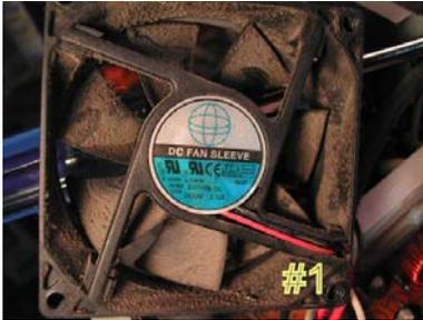
Cheap (Sleeve Bearing) fans die young. Bet on it. The cheaper the system, power supply, cooler, etc., the cheaper the fan. A cheap ball bearing fan may be just as bad. When you hear that sleeve bearing fan
