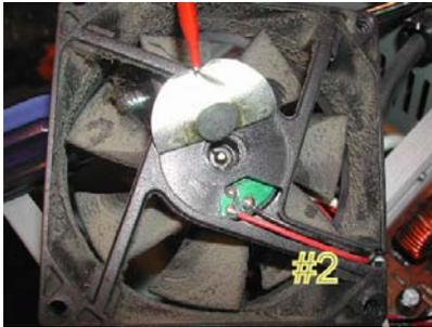
The better fans have a rubber plug that seals well and is almost invisible at times. The really cheap fans don't have a plug over the shaft area. If the fan still turns without much effort, just oiling it may make it well again. Apply a few drops of a good light machine oil such as, 3in1, Singer sewing machine, even ATF, but not the 30wt for your car engine, in the shaft hole.
